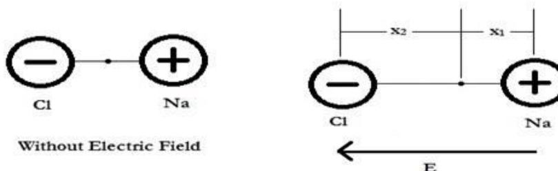
**Fig. Ionic polarization (a) unpolarized Ions (b) polarized Ions**
