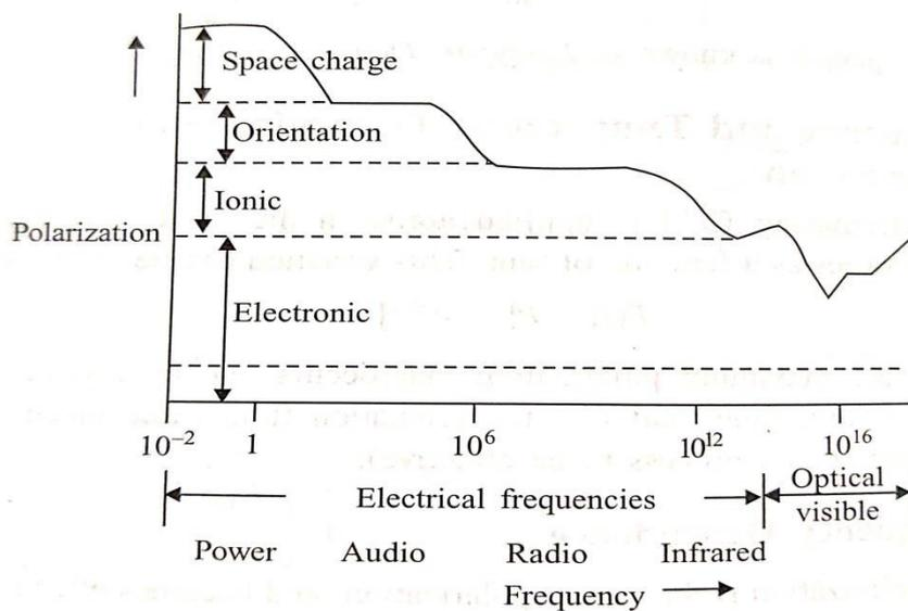
Frequency dependence on various polarization processes
