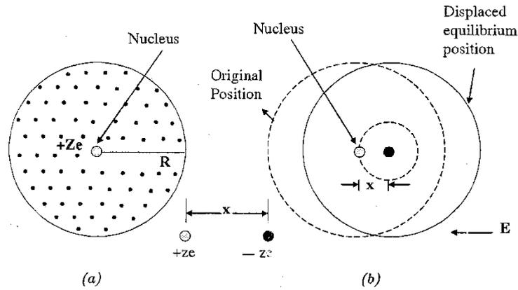
**Fig. Electronic polarization (a) unpolarized atom (b) polarized atom**
